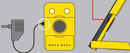
An empty WakaWaka needs about 4 hours to fully recharge using a micro-USB adapter.
