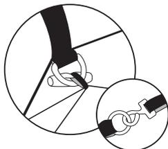
**4. NOW SPREAD OUT THE OUTER TENT** (grey). Also position the entrance first here and hang the outer tent on the airframe. To do this, secure the toggles to the D-rings at the top and the hooks to the O-rings at the bottom.
