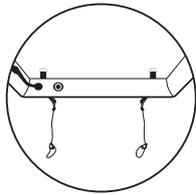
**2. TWO SEPARATE TIES** are secured to one of the struts. This is the entrance. Position this point where you want it.
