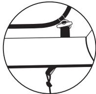
**3. NOW, STARTING FROM THE GRID**, you can begin to couple the inner tent to the grid. To do this, spread out the inner tent (white/blue) and position the inner tent entrance at the strut mentioned above. Now connect the toggles of the inner tent bottom (blue) to the black D-rings on the frame struts. Simply push through and twist and that's it!
